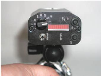
Lubricate until the dB level drops to the baseline.
