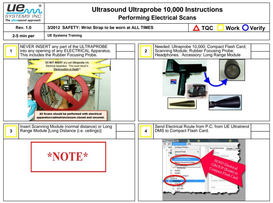
Page 1 of 4 \*Compact Flash Card & Module Inserted Before Turning Ultraprobe On\*
