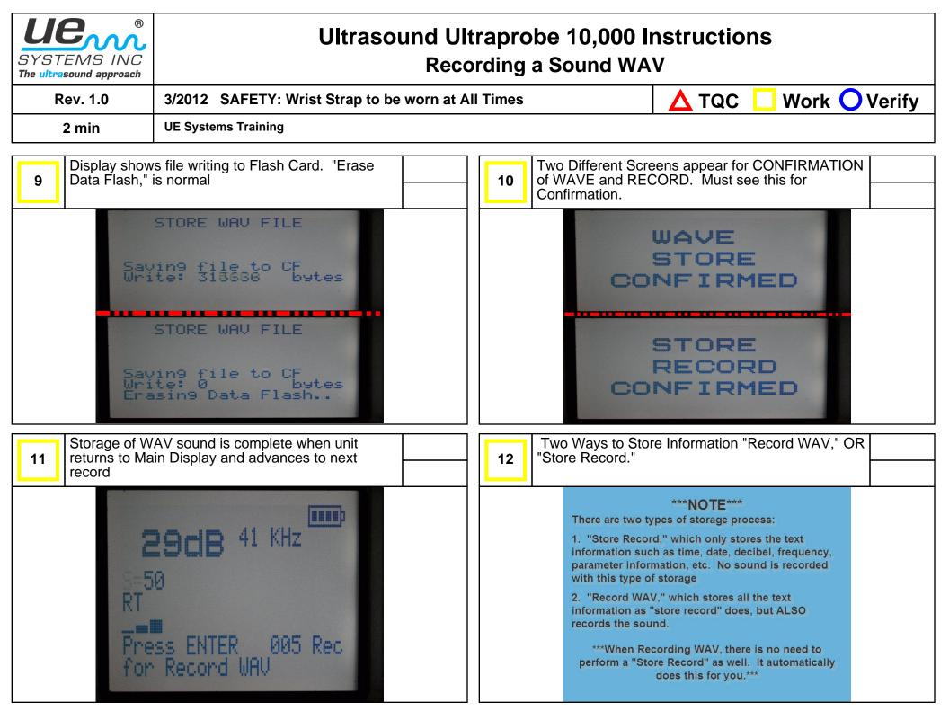
\*Compact Flash Card & Module Inserted BEFORE Turning ON\*
