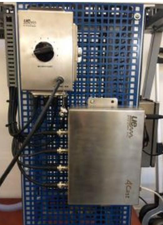
The 4Cast can connect to four bearings.
