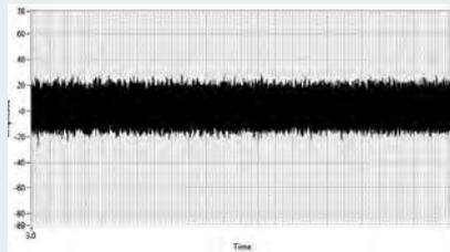
Figure 6 Time Waveform of another 2000KVA transformer in the same facility showing normal ultrasonic noise for this type of transformer
