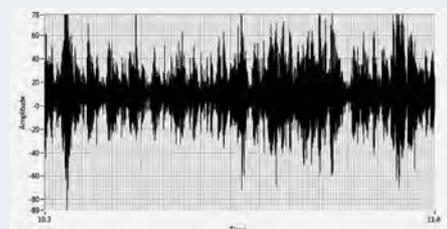
Figure 9 Time Waveform view of the recorded ultrasound of this contactor show distinct signs of severe tracking and early stages of arcing
