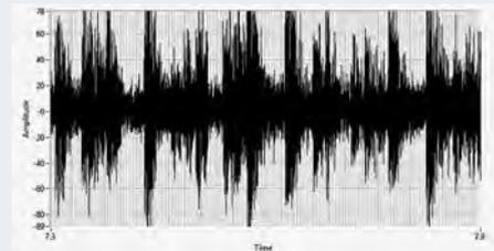
Figure 5 Time Waveform of recorded ultrasound from this transformer showing characteristics of arcing
