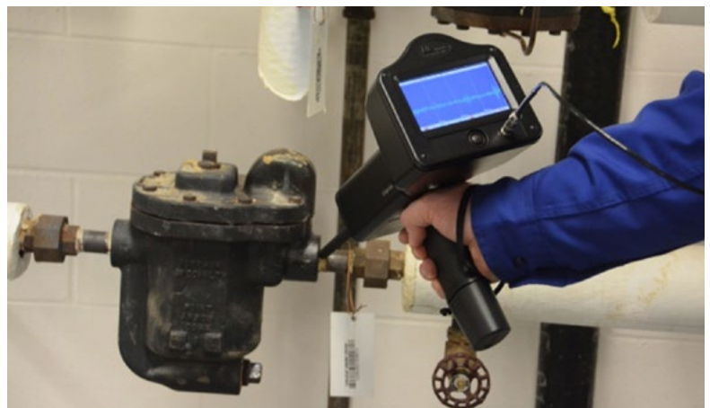
Figure 2 Inspector performing steam trap inspection on plant steam system using the UE Systems Ultraprobe.
