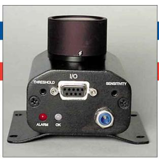
The UE-ECM 586 continuously monitors enclosed electrical equipment for the onset of corona, tracking and arcing. Utilizing a 0-10 VDC or a 4-20 mA output proportional to the received signal and a heterodyned output, it will warn in real-time as soon as any of these conditions happen.
