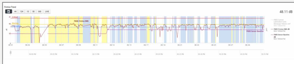
Figure 1B - Exhaust Fan Non-Drive End Bearing Friction (Ultrasound) Trend. The blue vertical bars indicate lubrication events, showcasing how friction levels fluctuate in response to each lubrication instance.
