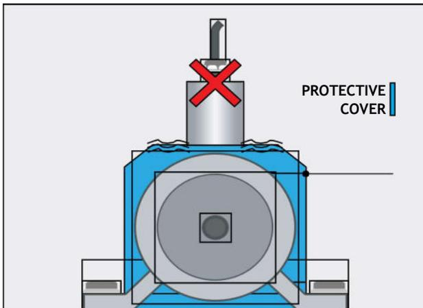
This sensor is placed on the protective cover and should not be used. It should be moved to a location on the machine housing that would allow for the most direct path of sound transmission from the bearing to the sensor.
