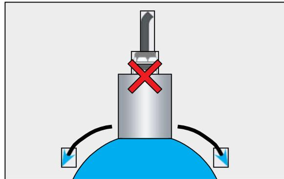
The sensor is placed at a location with debris that is not allowing the sensor to fully contact that machine housing and/or firmly attach to it. The surface should be cleaned of all debris before placing the sensor to ensure there is instability or weakness in the readings coming from the bearing.
