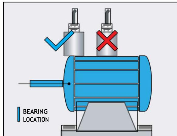
Both sensors are mounted vertically but the right sensor is not mounted as close as possible to the bearing and should not be used. The left sensor on the other hand is mounted in an acceptable location on the machine housing that is closest to the bearing.
