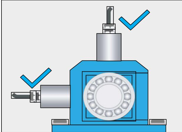
Both sensors are mounted vertically but the right sensor is not mounted as close as possible to the bearing and should not be used. The left sensor on the other hand is mounted in an acceptable location on the machine housing that is closest to the bearing.
