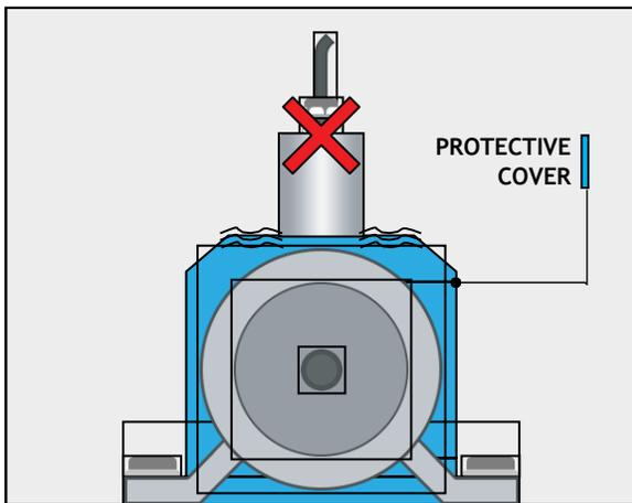
This sensor is placed on the protective cover and should not be used. It should be moved to a location on the machine housing that would allow for the most direct path of sound transmission from the bearing to the sensor.
