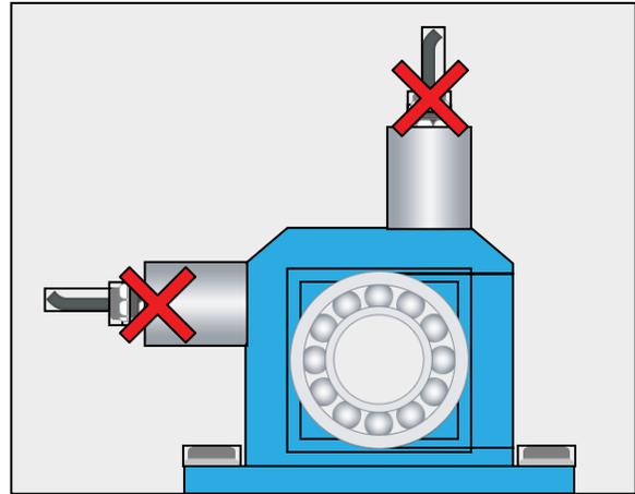
Both sensors are placed in locations furthest away from the centerline of the bearing and are not optimal for data collection
