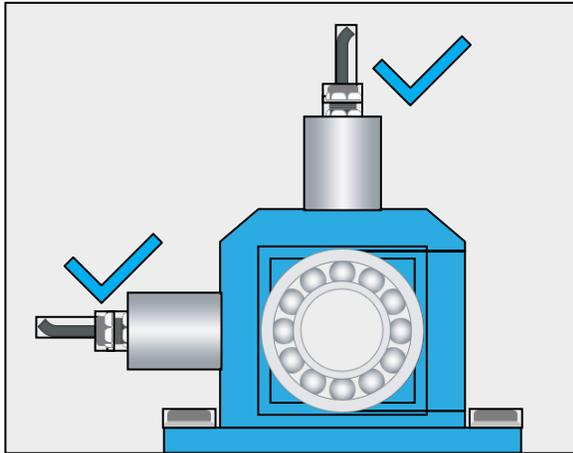
Both sensors are placed directly in line with the center of the bearing and are the shortest distance to it. Both the horizontal and vertical locations are acceptable, and either location can be used.
