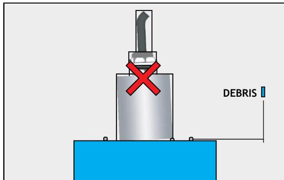
The sensor is placed at a location where it has limited surface contact area and is prone to rocking and movement side to side. This lack of stability will cause the readings to be inconsistent and potentially erroneous in nature and should not be used.
