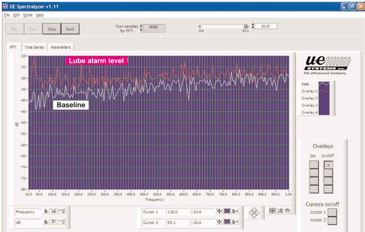
Fig. 1. The lube alarm level indicates a need for lubrication. The baseline shows when application is complete.
