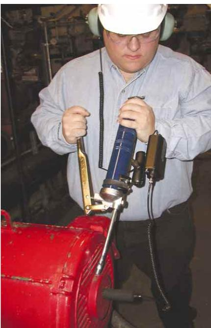
*Fig. 2. As an operator lubricates, there is a visual and audible indication when lubrication is completed.*
