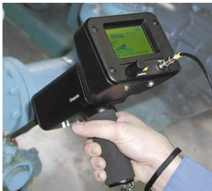
Ultrasonic technology is sound-sensitive and can spot numerous leaks.
