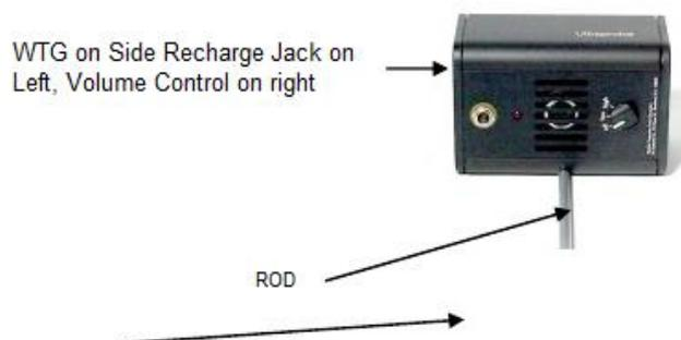
7. Place the rod in the middle of the transducer are (as above)
