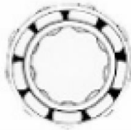
Lack of Lubrication Increases amplitude levels
