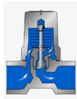
Should the bellows in a bellows trap become compressed by water hammer, the trap will not function properly. The occurrence of a leak will prevent the balanced pressure action of these traps. When either condition occurs, the trap will fail in its natural position either opened or closed. If the trap fails closed, condensate will back up and no sound will be heard. If the trap fails open, continuous rushing of live steam will be heard.
