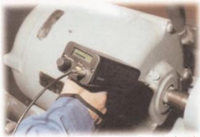
*Checking grease levels using ultrasonic leak detector.*
