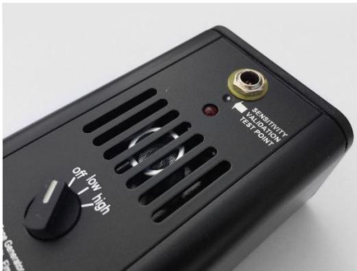
The WTG 1 Tone Generator is an ultrasonic transmitter designed to flood an area with ultrasound. This Tone Generator is a WARBLE TONE GENERATOR. This internationally patented transmitter sweeps through a number of ultrasonic frequencies in a fraction of a second to produce a strong, recognizable "Warble" signal. The warble tone prevents a standing wave condition, which can produce false readings. This is typically used for Sensitivity Validation.
