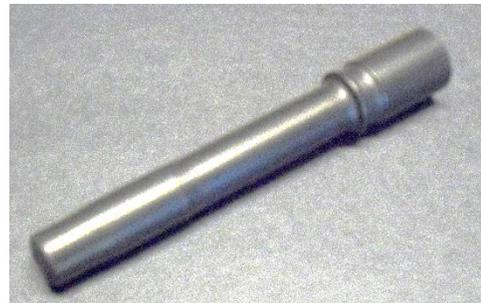
**STETHOSCOPE EXTENSION KIT.** This consists of three metal rods that will enable a user to reach up to 31 additional inches (78.7 cm) with the Stethoscope Probe.
