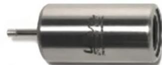
**STETHOSCOPE (CONTACT) MODULE.** This is the module with the metal rod. This rod is utilized as a "waveguide" in that it is sensitive to ultrasound that is generated internally such as within a pipe, bearing housing or steam trap. Once stimulated by ultrasound, it transfers the signal to a piezoelectric transducer located in the module housing directly behind the "wave guide". For placement align the plug with the corresponding receptacle in the front end of the pistol housing and plug in.
