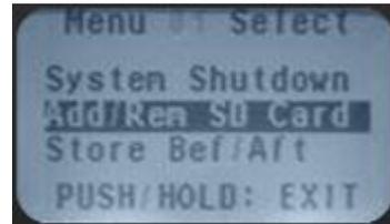
**MENU 02 STORE BEFORE/AFTER.** When selected, this function allows the user to store decibel readings before adding lubricant and after adding lubricant.
