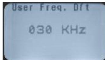
**MENU 08 FREQUENCY ADJUST.** This feature allows the user to change frequencies between 20 kHz and 100 kHz in one kHz intervals.
