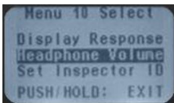
**MENU 10 HEADPHONE VOLUME.** This feature allows for adjustments to the sound level or volume level in the headphone. Click to enter the volume selections range from 0% to 99%. The default value is 95%.
